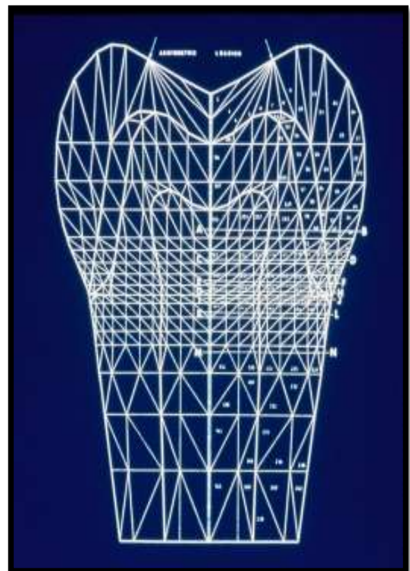
Figure 19: Axisymmetric Finite Element Model with Three Marginal Configurations
