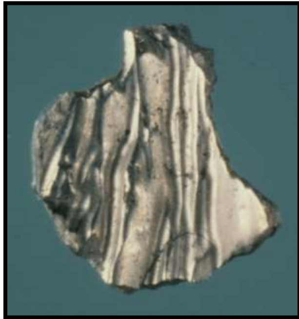
Figure 4: Luder Lines in Amalgam Due to Stress
